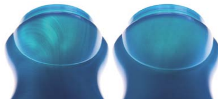
Roll-on housing molded without Promix Static Mixer
