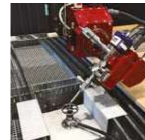
EDGE 5 Calibration Automatic 5 Axis Calibrating System by a special NC test routing and device
