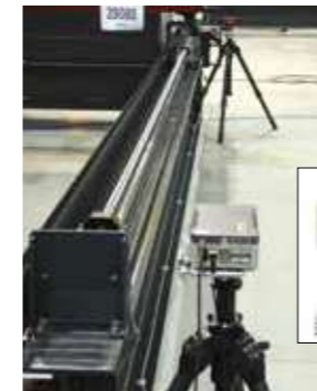
Renishaw Laser Straightness inspection and verification
