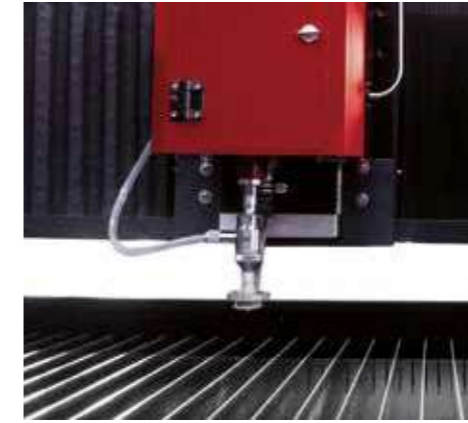
Touch probe Sensor with Anticollision, Laser Pointer, and Vacuum Assist Tastatore con Anticollisione, Laser e Vacuostato
