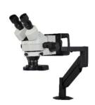
Stereo binocular microscope with shutter generator unit driven / Adjustable magnification from x4 to x20 / Cold lighting ring with 60 white light LEDs - Strong and focused illumination with shadow free - The 60 lights are divided into 4 individual zones. Each zone has its independent ON/OFF control as well as brightness control. Is including one set of 2 ergonomic foam wrist/hand/arm supports.
