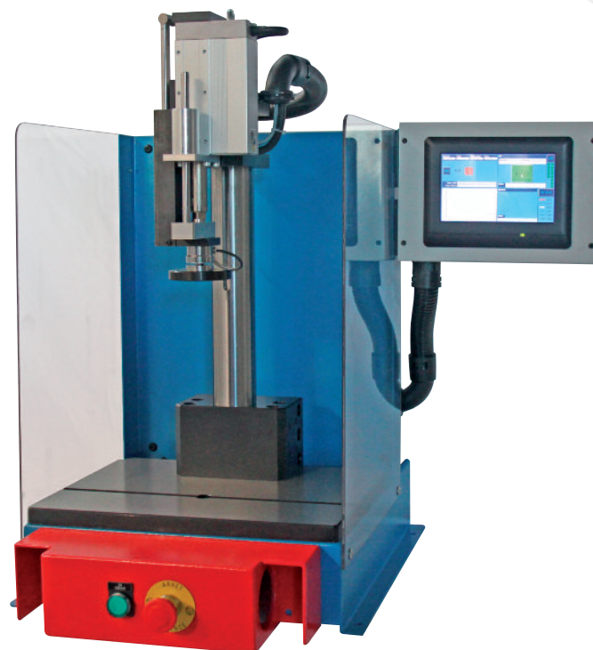
Electric press equipped with a force and a displacement sensor, associated with the process controller and an 8" display terminal.
