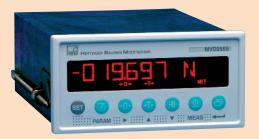
3 - System for measuring force and displacement with analysis by envelope curve. The programming is carried out by a PC using the software provided by EMG.
