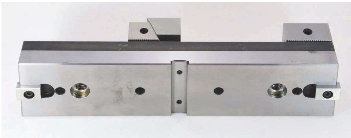
PSE clamping rail 320 mm prepared with notches 16 H7 mm and fitting bores \varnothing 25 H7 mm screwing through T – notch 4 times distance 80 mm for M8 screws
