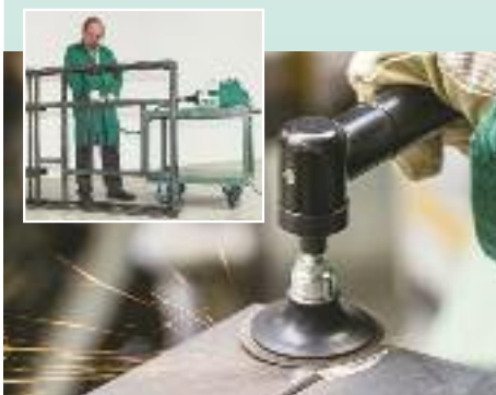
Smoothing weld seams 2
