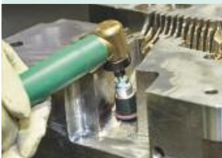
Levelling milling grooves
