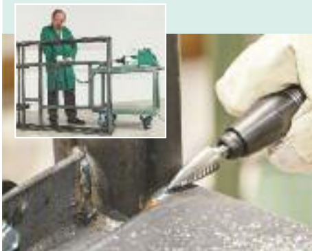
Smoothing weld seams 1
