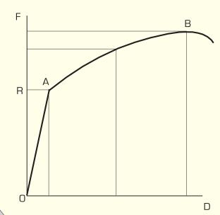
In the area **OA** of the graph the elongation is small and proportional to the effort. (Hooke's Law) Point 'A' on the graph is known as the elastic limit. This is the point where once the effort reaches a level 'R' and then is released the steel bar returns to its initial length. (No permanent deformation)
