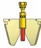
GF FITTING SWIVEL Compression Cross-Section View
