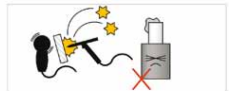
9. For mold lapping and polishing, exercise caution against the adhesion of welding sparks, scraps, metallic contaminants, etc.
